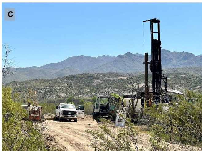
A - General topography at Basin, Sonic drill rig in foreground B - Typical Basin project stratigraphy, Tuffs overlying clay formations C - Boart Longyear sonic drill rig in action drilling hole BES-23-04 D - Clay horizon core from current drill programme
