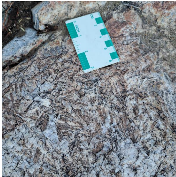
Figure 12: Weathered fine-medium grained spodumene
