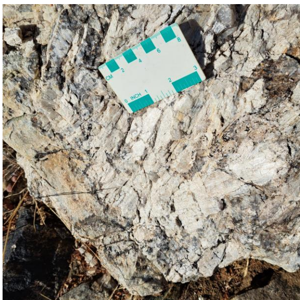
Figure 11: Coarse grained Spodumene
