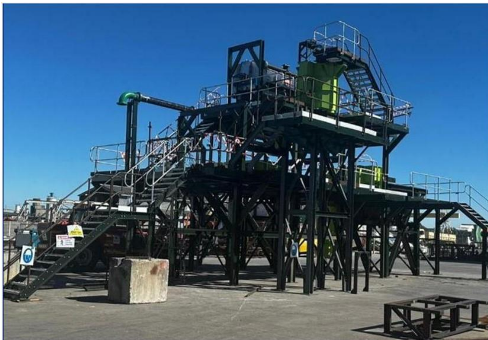
Figure 7 – A typical spodumene DMS plant – a small modular footprint & simple process Below is the actual DMS plant for Atlas Lithium's Neves assembled prior to shipment – 1.1Mtpa ore throughput, 2-stage DMS, 146ktpa SC5.5 concentrate
