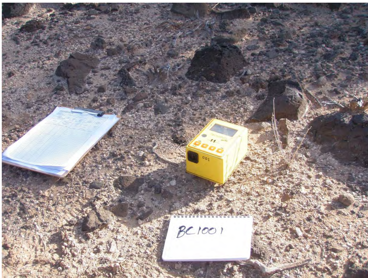
Figure 9-2: A Tromino Mobile Passive Seismic Surveying Instrument
