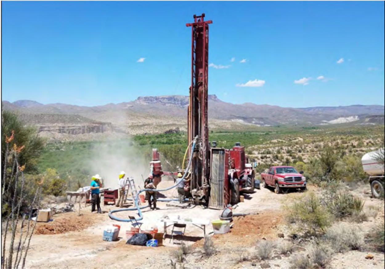
Figure 10-2: RC Drilling in progress on hole BCRC18-10
