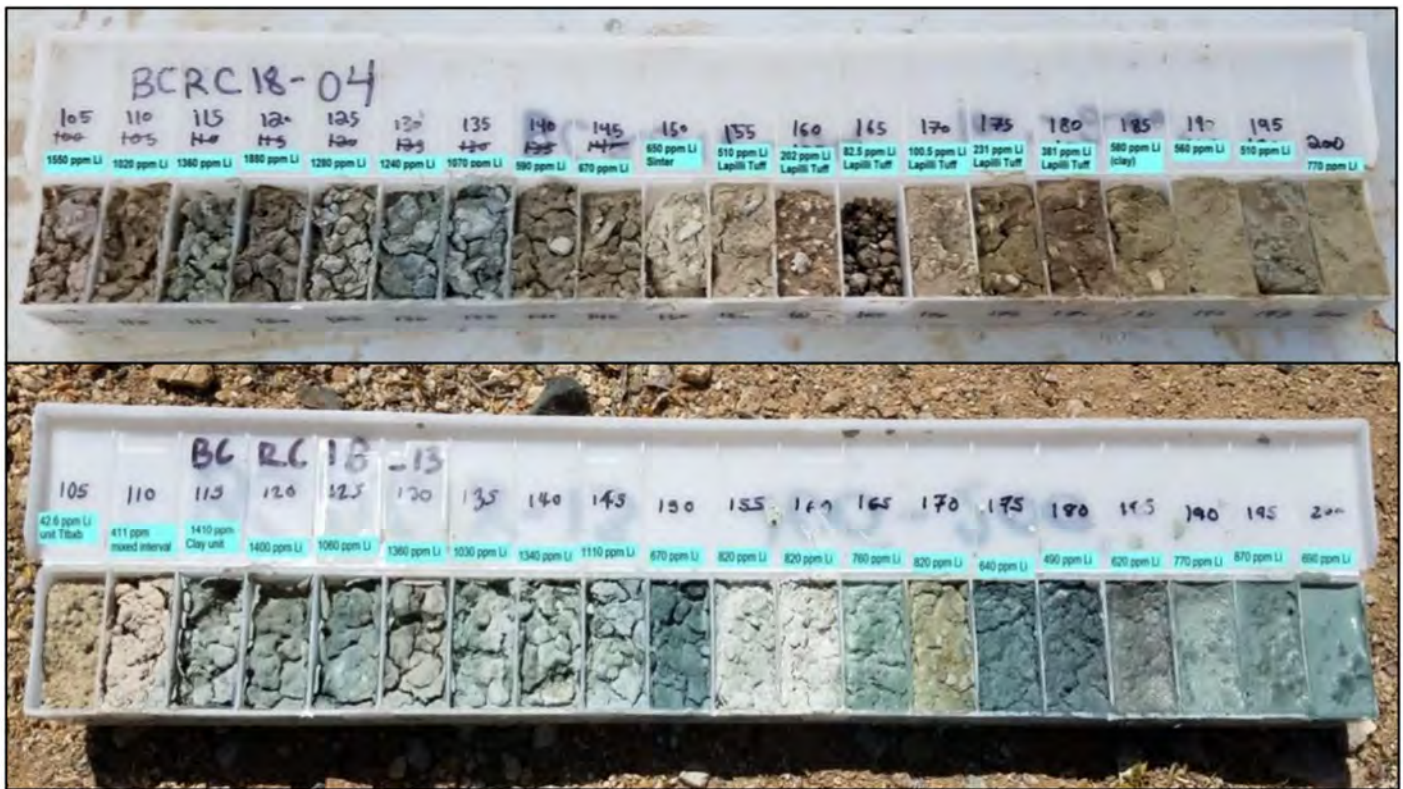
Figure 7-2: RC Chip Samples from BCRC18-04 and BCRC19-13 Showing Li Grades in Permanent Marker
