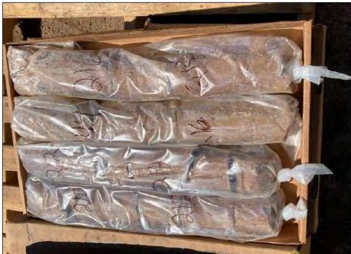
Figure 10-5: Wax Coated Box Containing Sonic Drill Core
