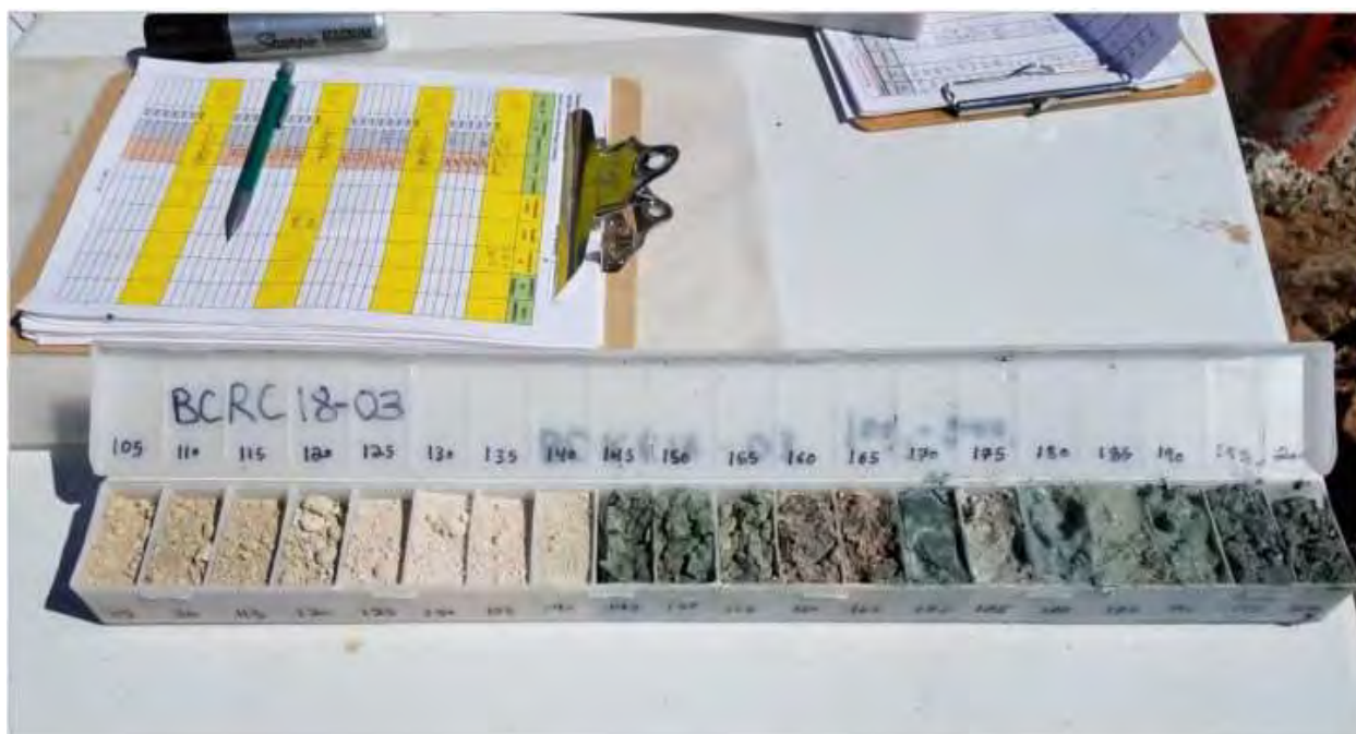
Figure 10-3: An Example of an RC Chip Tray
